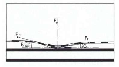
Fig. 2: Linear shear forces occurring in overlaps of bitumen sheets
